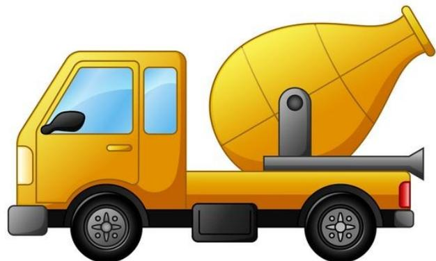
Concrete is brought to the construction site by mixer trucks. The concrete is carried in a big drum, which keeps turning to stop the cement from setting hard.
